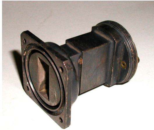
British to American waveguide matching transformer. Note also the different union on each type.
