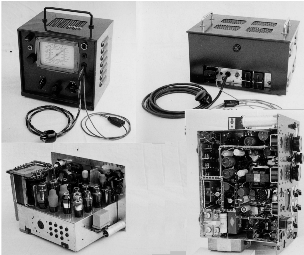
Radio tuner, Pre Amplifier, and 20 Watt audio amplifier all homebuilt.
